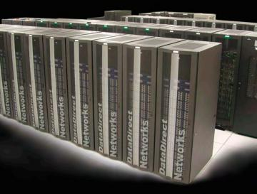
file system that eventually will serve all the NCCS systems. It will connect to the InfiniBand and Ethernet internal networks. Because all simulation data will eventually reside on Spider, users will not need to transfer files among multiple computers and data management systems.
