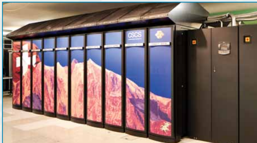
Monte Rosa, the Swiss National Supercomputing Centre’s 402-teraflop XE6 Cray supercomputer, uses only CPUs. The entire computational-science community benefits from efforts to optimize CPU performance. Image credit: Michele De Lorenzi/CSCS
