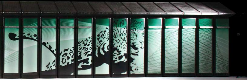
The new 1.64-petaflop Cray XT Jaguar features more than 180,000 processing cores, each with 2 gigabytes of local memory. The resources of the ORNL computing complex provide scientists with a total performance of 2.5 petaflops.
