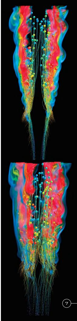
flames can blow out. For flames to stabilize, or continue to burn downstream from the burner, turbulence, which mixes fuel with air to enable burning, must exist in balance with key ignition reactions that occur upstream of where the flames appear.
