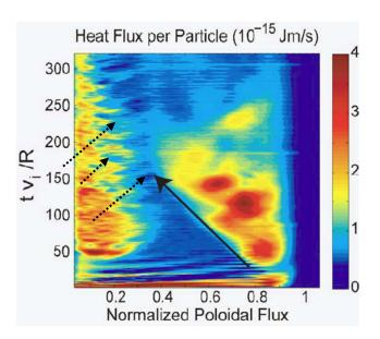
Fig. 17. Heat flux contour in the global space-time space, exhibiting the out-to-in propagation of the turbulence front.
