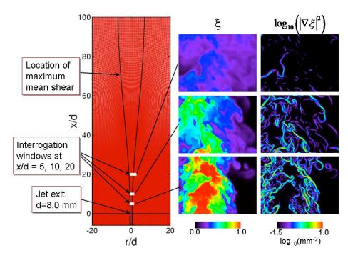
**Fig. 25.** Cross section of the computational domain showing key features of the grid topology. The domain includes the entire burner geometry, as shown in Fig. 23. To the right are single-shot measurements of mixture fraction and scalar dissipation. The jet Reynolds number is 15,200.
