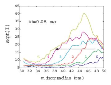
Fig. 14. Inward propagation of the square root of turbulence intensity Sqrt(I) during the bursty nonlinear period, where  $I = \langle (\delta \varphi) 2 \rangle$ . Each plot is drawn in 0.08 ms interval, and the total propagation time is only 0.4 ms.
