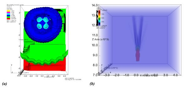
Fig. 5. (a) Extraction of radiation dose contours and (b) a volume rendering from the nuclear power plant simulation from the Denovo code. Q4
