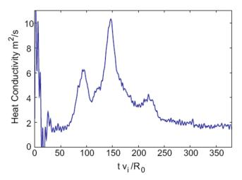
Fig. 19. Time behavior of effective ion thermal conductivity (thermal flux divided by local Ti gradient) from the start of the simulation across  $\psi N = 0.64$ , which corresponds to r = 42 cm on the outside midplane. The self-organizing process is bursty.
