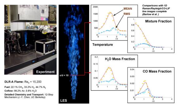
**Fig. 24. Baseline flame used for problem scaling.** (*left*) Photograph and (*center*) corresponding LES of the DLR-A flame. (*right*) Representative comparisons between experimentally measured (symbols) and modeled (lines) results showing acceptable agreement.
