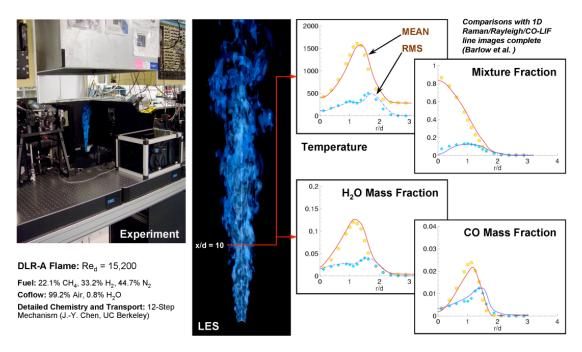
Fig. 26. Comparison of experimentally measured (symbols) and modeled (lines) results showing acceptable agreement.
