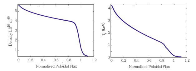
**Fig. 10. Early-time plasma density and temperature profiles.** Electron temperature is assumed to be equal to ion temperature. Notice that the temperature pedestal knee is located at a somewhat smaller minor radius than the density pedestal knee, making the relative temperature slope high between the two knees.
