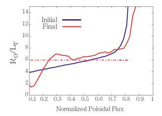
Fig. 18. Self-organizing modification of the background temperature profile by the incoming turbulence. The horizontal line represents the nonlinear criticality in the core plasma.
