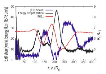
Fig. 20. Phase relation between the temperature gradient, heat flux, and E×B shearing dynamics at a radial location.
