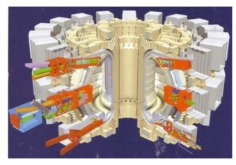
Fig. 8. Schematic of the ITER tokamak, where the first wall of the innermost structure of the device is shown, with the divertor chamber at the bottom. For more information, see www.iter.org.
