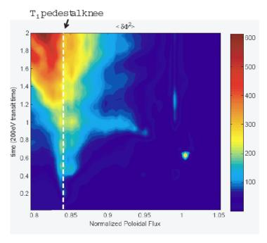
Fig. 15. An enlarged image of the turbulence intensity  $< |\delta \varphi|^2 >$  contour in the radius-time space in the pedestal area.
