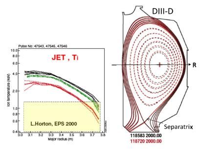
Fig. 9. (*left*) Nonlocal nature of the ion temperature (T<sub>i</sub>) profile. As the edge T<sub>i</sub> increases, the core T<sub>i</sub> increases together in a stiff shape. (*right*) The cross section of DIII-D magnetic surface inside the first wall. Open and closed magnetic surfaces are shown, with the magnetic separatrix surface in between. For more information on the DIII-D device see http://web.gat.com/global/DIII-D.
