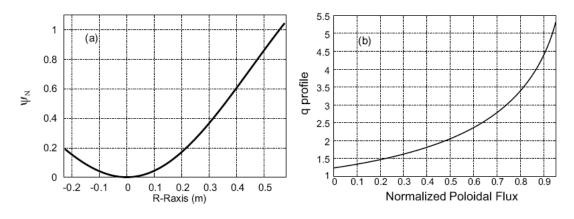
Fig. 12. (a) Relationship between the normalized poloidal flux  $\psi N$  and real distance in meters from the magnetic axis (Raxis = Ro) to the flux surface (R) along the midplane. (b) Radial profile of the safety factor q.
