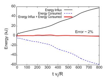
Fig. 21. Energy accounting within  $0.3 \le \psi N \le 0.7$  between the total influx across the inner boundary (black curve) and the sum of the consumed energy (blue curve) to the particles, the electric field, and across the outer boundary. Red line shows sum of black and blue curves. About 2% error is noticed.
