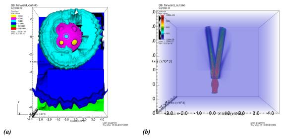
Fig. 4. (a) Extraction of radiation dose contours and (b) a volume rendering from the nuclear power plant simulation from the Denovo code. Q2
