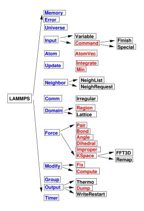
Figure 1: Class hierarchy within LAMMPS source code.
