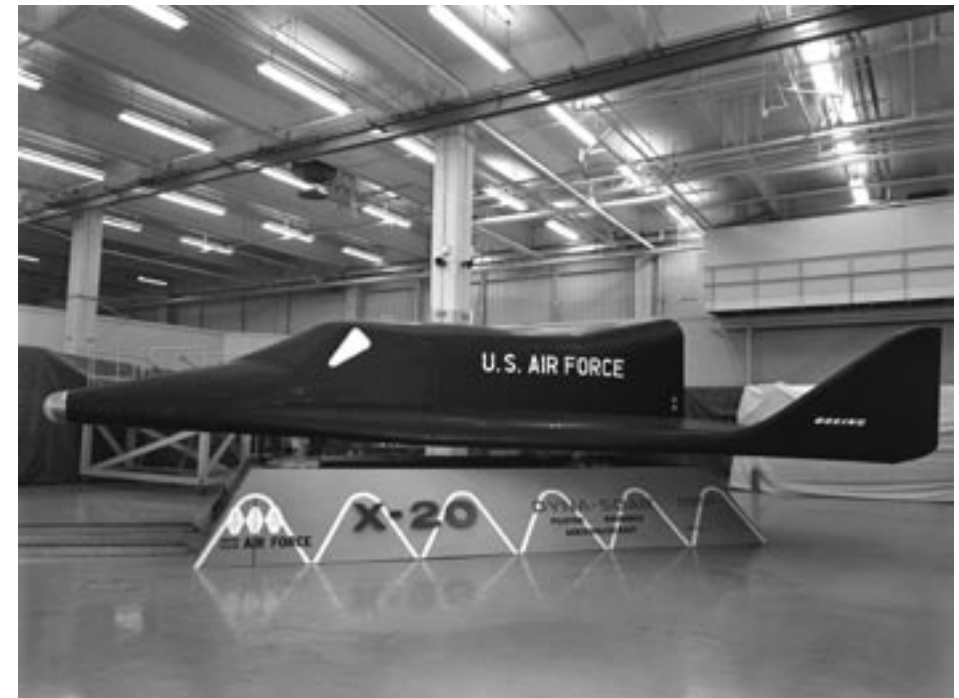
Full-scale model of Dyna-Soar, on display at an Air Force exhibition in 1962. The scalloped pattern on the base was intended to suggest Sänger's skipping entry. (Boeing Company archives)
