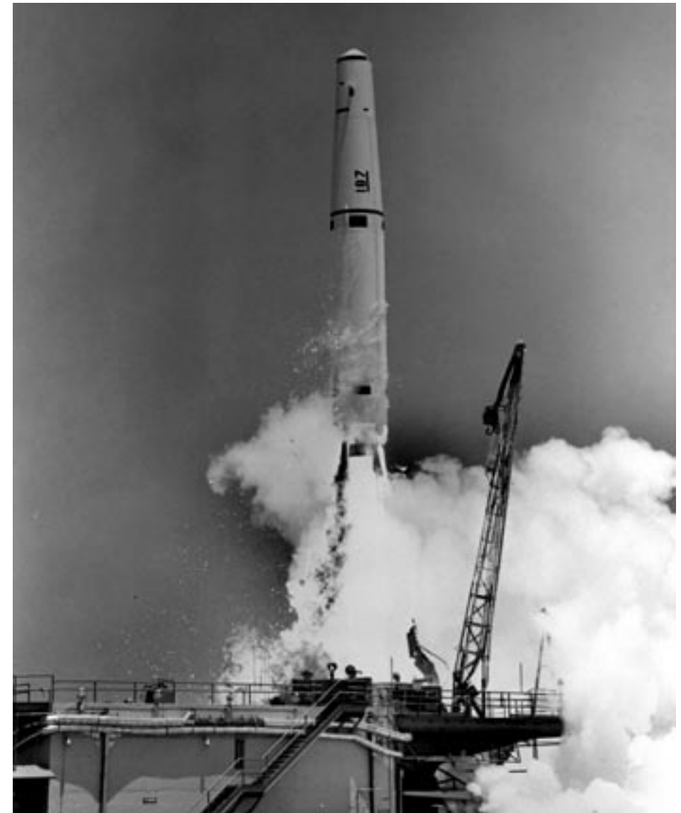
Thor missile with heat-sink nose cone. (U.S. Air Force)
