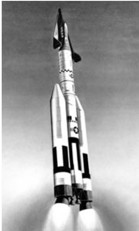
Artist's rendering showing Dyna-Soar boosted by a Titan III launch vehicle. (Boeing Company archives)
