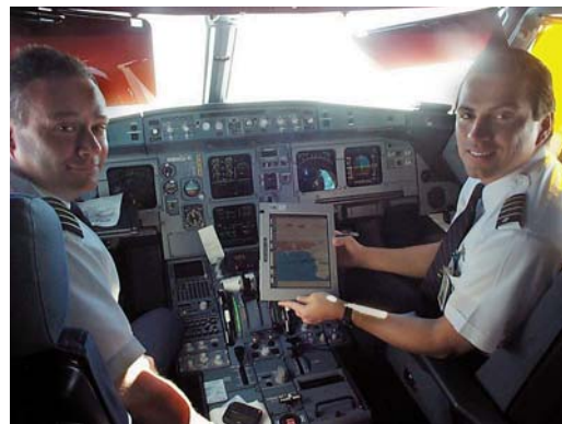
Figure 4. Data-link weather display on tablet computer in cockpit of United Airlines A320.
