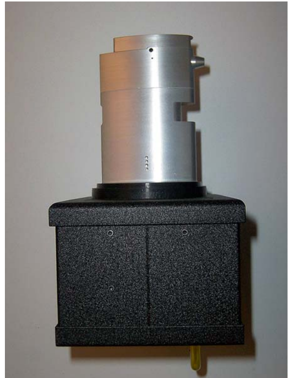
Figure 13. TAMDAR sensor showing probe body (top) and attached signal processor unit (box at bottom).
