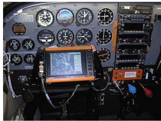
Figure 2. Prototype of AWIN display mounted to yoke of NASA C-206 research airplane.
