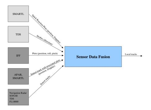
Figure 4: Input data of the Sensor Data Fusion
