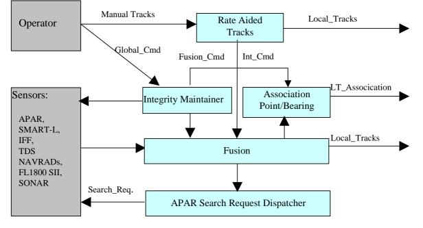
Figure 3: Tasks of Sensor Data Fusion
