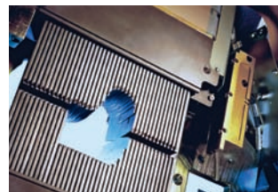
Multileaf collimator with movable leaves
