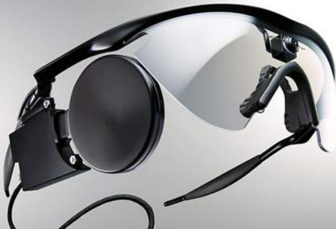
The Argus II or the "bionic eye" for people suffering from degenerative retina disease.
