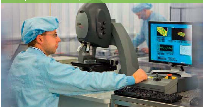
Hendrik Specht examines the surface form of a micro sensor on a white light interferometer in a laboratory at the Fraunhofer Institute ENAS in Chemnitz. This type of analysis is also a means of monitoring the quality of future sensory micro and nano systems.
