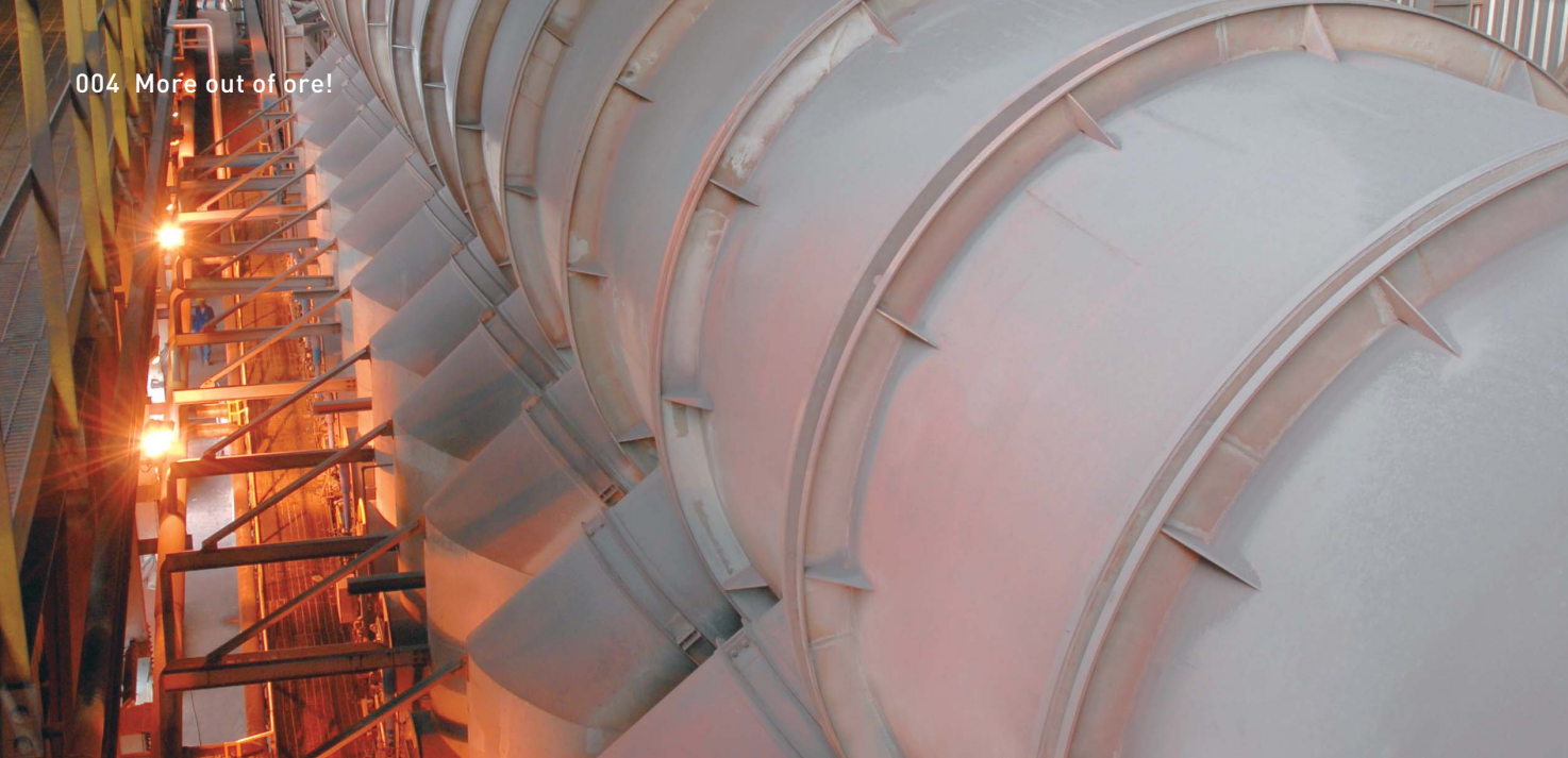
Indurating furnace at CVRD's Sao Luis pelletizing plant in Brazil.
