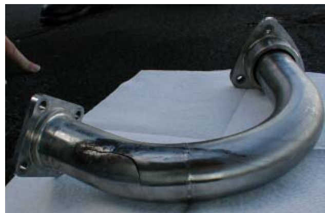
Figure 4 Fuel Pipe Crack & Scratches
