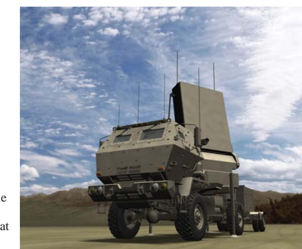
This artist's concept shows the Lockheed Martin EQ-36 Counterfire Target Acquisition Radar. This system will provide U.S. Army soldiers with the capability to detect, classify, track and determine the location of enemy indirect fire such as mortars, artillery and rockets.
