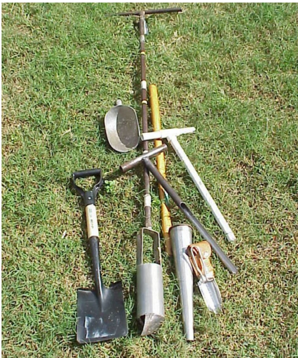
Figure 4. The collection of soil samples for nematode analysis can be acquired from the field using either cylindrical sampling tubes, trowels, bucket auger, or shovel.
