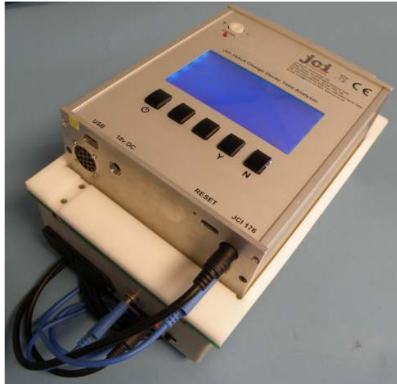
JCI 155v6 Charge Decay Test Unit
