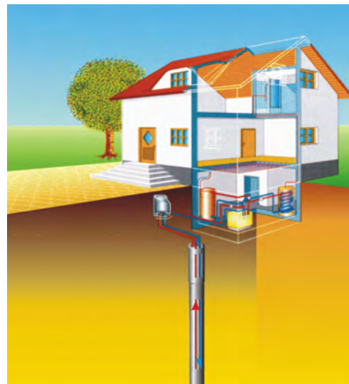
Fig. 8.29 Vertical borehole heat exchanger system (after [1999Ano a ; yellow box in building basement: heat pump).
