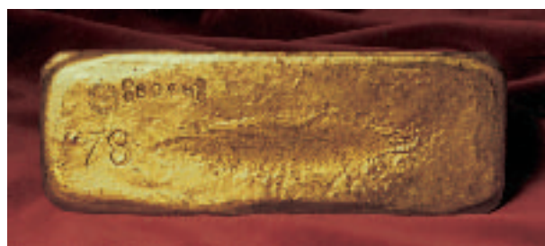
A gold ingot weighs 12.5 kilos on average. It is not square, but slightly wider at the bottom than at the top
