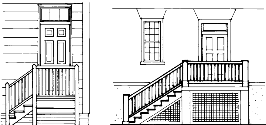
Figure 95. Details of entrance stoops.
