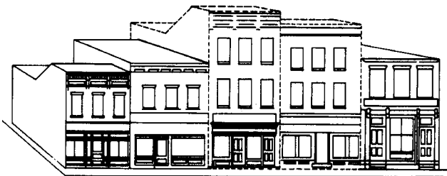
YES A successful example of a large building broken down into two "building elements." (Sketches courtesy of Vivian P. Hopkins)
