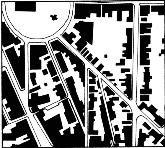
Figure 57. Partial plan of the historic district street intersections. Triangular and other unusual-shaped lots were created by the intersection of radiating streets with other streets. At all street intersections buildings should follow the property lot in order to reinforce the town plan.
