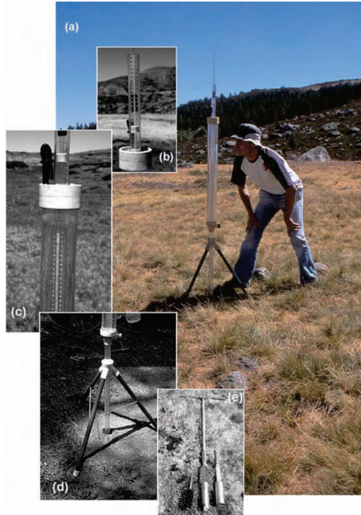
Figure 5. The constant-head well permeameter: general view (a), well head scale (b), water reservoir (c), tripod (d) and soil auger set (e).
