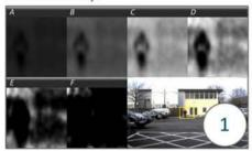
In the above image the person was at a distance of 25m from the T5000. The change in contrast around their torso indicates the presence of a concealed object.
