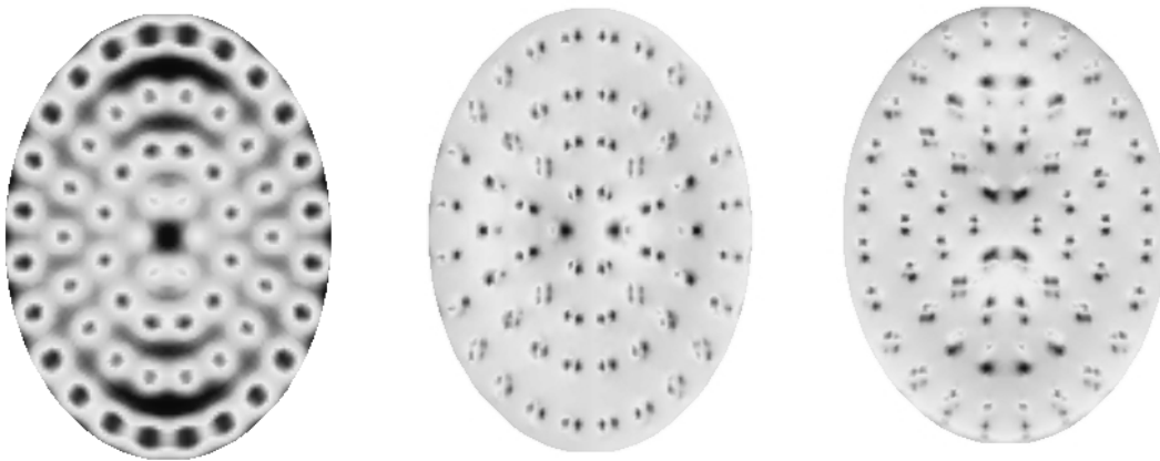
Figure 10. Support print-through in Z gravity loading (left, 20 nm), and lateral loading in X and Y (right, both 1 nm RMS).
