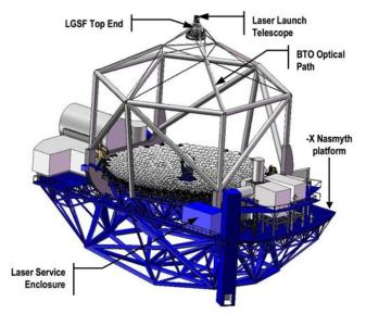
Figure 1: Original (2006) LGSF Conceptual Design
