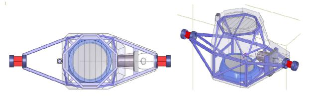
Figure 6: Top view (left) and isometric view (right) of the LLT mounted in its space frame, with two flexures along the input optical axis.
