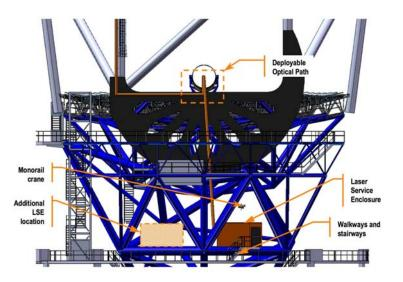
Figure 10: Location of the LSE within the telescope azimuth structure
