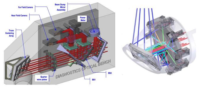
Figure 8: Diagnostics Optical Bench
