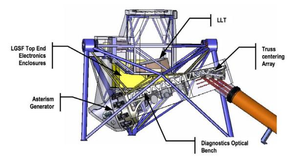
Figure 3: LGSF Top End in zenith pointing orientation as viewed from behind the telescope
