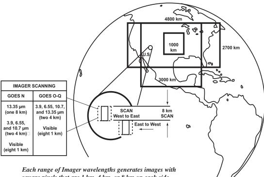
square pixels that are 1 km, 4 km, or 8 km on each side. For instance, images produced at wavelengths of 10.20 -11.20 micrometers (µm) have pixels that are 4 km (2.5 miles) on each side. A smaller number of pixels indicate better-quality images. Note that the resolution for the 13.00 - 13.70 µm wavelength changes for GOES-O-Q.
