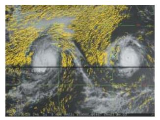
This image shows low-level visible clouddrift winds around hurricanes Eugene and Dora. Three 15-minute sectors (above the horizontal black line) and three 30-minute sectors (below the black line) were used to derive the visible winds from Imager data. Note the significant improvement in detail of the wind field from data that was obtained in 15-minute intervals in the top half of the image. The straight end of each wind barb points in the direction that the wind is blowing.
