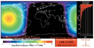
Absorption of highfrequency radio waves in the D-Region of the ionosphere (the lowest layer of the ionosphere) is directly affected by the level of solar x-ray flux. The D-Region absorption product was developed to assist high-frequency radio operators and is based entirely on real-time data from the x-ray sensor.
