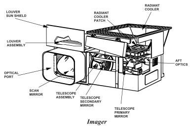
The Imager simultaneously senses emitted thermal and reflected solar energy from selected areas of the Earth. It uses a scan mirror system to alternately sweep east to west and west to east perpendicular to a north-to-south path. The rate of scanning allows the instrument to gather data in its five spectral channels from a 1,864 x 1,864-mile area (3,000 x 3,000 km) in three minutes and from an area of 621 x 621 miles (1,000 x 1,000 km) in just 41 seconds.
