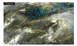
Wind data is derived from the GOES Sounder's water vapor channels in the mid-troposphere, the level of the atmosphere where the jet stream develops and carries weather systems. The straight end of a wind barb points in the direction that the wind is blowing. The density of a barb's tail shows the intensity of the wind. The color of a barb shows its altitude.
