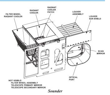
Detecting conditions that may lead to severe storms is one major function of the Sounder. Data collected by the instrument is processed on the ground so that it generates a numerical designa-
