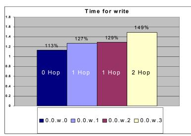
Figure 5. Write-Only Thread Running on Node 0, Accessing Data from 0, 1 and 2 Hops Away on an Idle System
