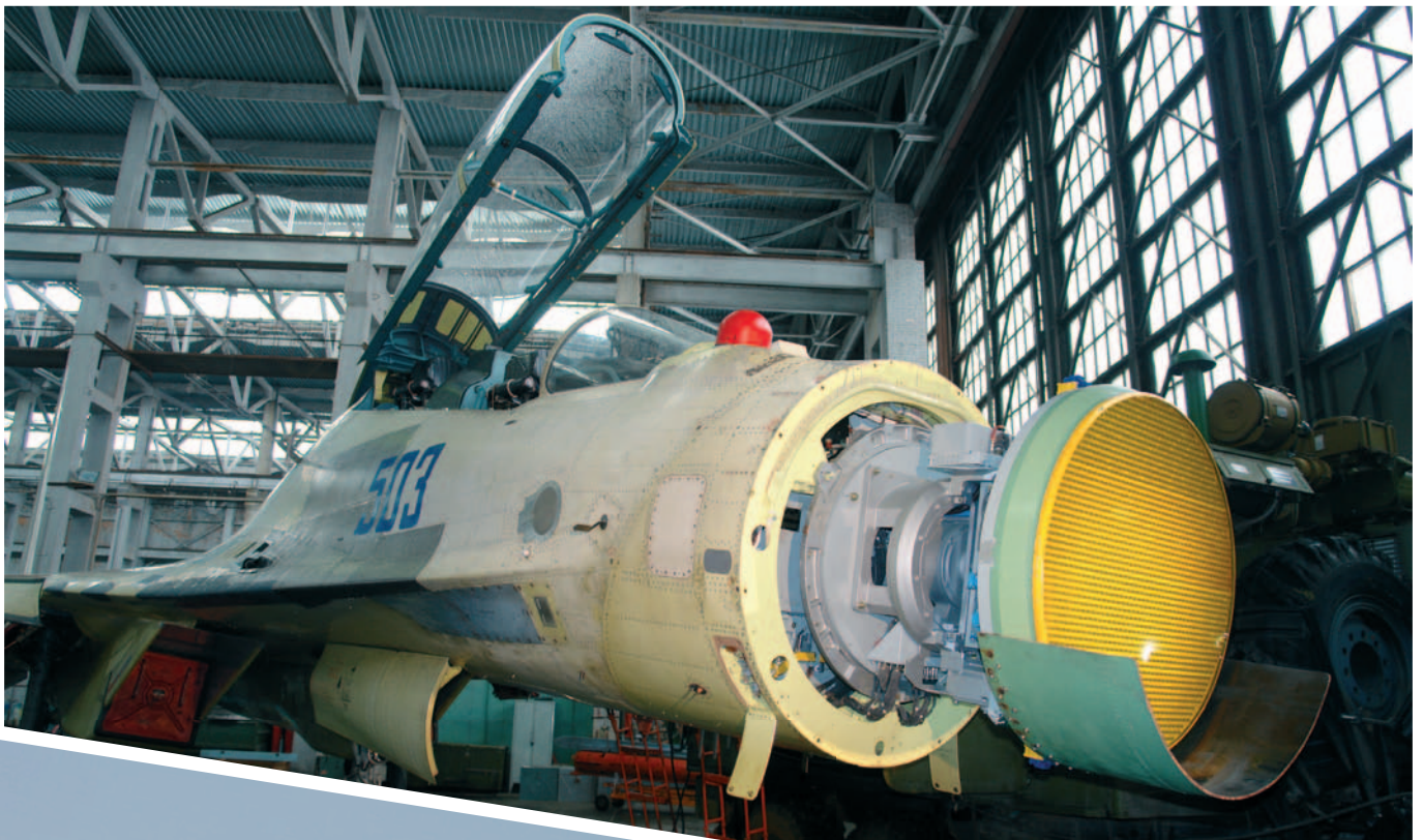
Irbis-E phased-array radar is being tested onboard the Su-30MK2 No 503 flying testbed since early 2007
