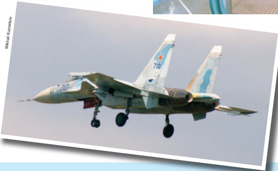
NPO Saturn 117S turbofan unveiled at MAKS 2005 was tested onboard Su-27M No 710 flying testbed in 2004-2006
