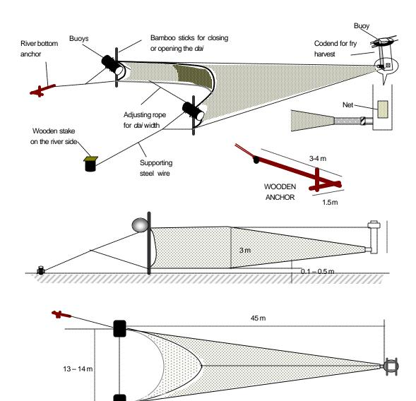
Figure 8 Bagnet or *dai* for catching Pangasiid fry, as used in Cambodia and Viet Nam.
