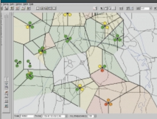
Fig. 4 Cell modeling using Voronoi polygons - Alcatel 956 RNO
