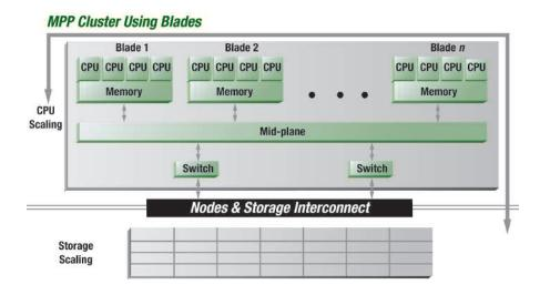
A number of vendors offer data warehouse solutions based on blade technology. In a typical scenario, each blade functions as an SMP cluster of processors and shared RAM, within a matrix of blades operating in parallel. This amounts to a tightly consolidated version of the MPP on clustered SMP architecture described earlier.
