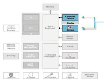
ST's advanced family of Integrated Passive and Active Devices now includes the "VID" series EMI filters. Based on IPAD™ technology, they offer the lowest line capacitance on the market along with superior EMI attenuation capabilities. "VID" series EMI filters are perfectly tailored for high data rate LCD displays and Camera interfaces in mobile phones.
