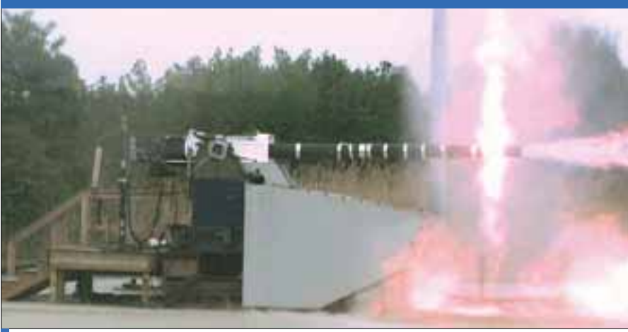
The US Army's Benét Laboratories is developing the XM360 lightweight 120 mm gun as the main Los/Blos armament for the MCS. Firing tests began at Aberdeen Proving Ground in November 2004. (US Army)
