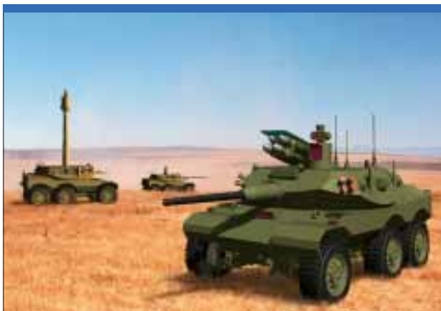
BAE Systems is leading the design and development of the Armed Robotic Vehicle. The ARV-RSTA (left) and the ARV-Assault ARV-A are designed to be controlled by troops on the ground or in manned ground vehicles. Under present plans each FCS brigade will include 45 ARVs. (BAE Systems)
