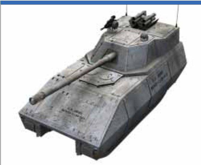
One of the largest technical challenges of the FCS project will be giving the 25-tonne General Dynamics Mounted Combat System (MCS) an equal or better level of survivability as compared to the 70-tonne M1A2 tank that it is intended to replace. (US Army)
