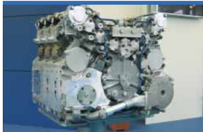
The Detroit/MTU engine will be a version of the MTU Series 890 V6 yielding up to 750 bhp with a maximum torque of 1235 Nm at 4250 rpm for a dry weight of only 470 kg. (Armada/EHB)
