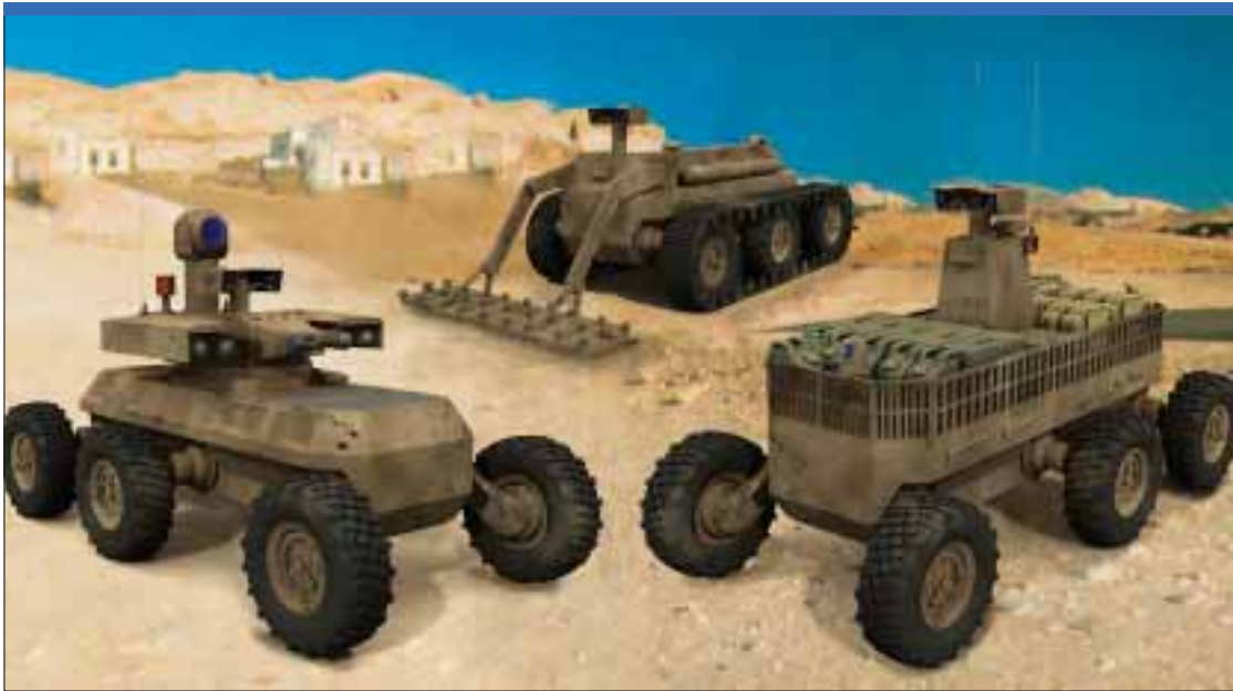
Lockheed Martin is developing the 6 x 6 Multifunction Utility/Logistics and Equipment (Mule) unmanned ground vehicle in three variants: the Armed Robotic Vehicle - Assault (Light) (left), a Countermine variant (centre) and the Transport Mule (right). The Mule's success is dependent upon an advanced 6 x 6 independent articulated suspension coupled to in-hub motors. (Lockheed Martin)
