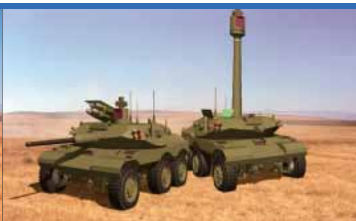
BAE Systems is leading the design and development of the Armed Robotic Vehicle. The ARV-RSTA (left) and the ARV-Assault ARV-A are designed to be controlled by troops on the ground or in manned ground vehicles. Under present plans each FCS brigade will include 45 ARVs. (BAE Systems)
