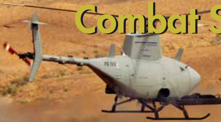
Northrop Grumman is developing the MQ-8B Fire Scout into the FCS Class IV drone
