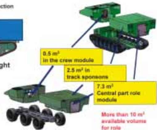
The basic platform weight is 9.5 tonnes allowing a further eight tonnes for the mission module, personnel and protection. Inside the mission module there will be 7.33 metres 3 of volume and a further 2.53 metres 3 in the sponsons on either side of the module. Both the wheeled and tracked variants fit inside a C-130. (BAE Hägglunds)
