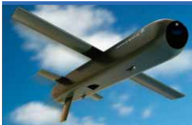
Powered by a turbojet engine and fitted with wings the Lam will have a cruise endurance of at least 45 minutes, enabling it to attack targets to a maximum range of about 200 km or loiter for about 30 minutes at a range of 70 km. (Lockheed Martin)
