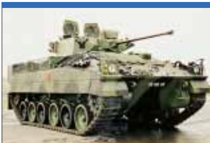
Under the Warrior Lethality Improvement Programme Technology the IFV is expected to be fitted with a new turret mounting the CTA International 40 mm Cased Telescoped Weapon System (CTWS). This weapon is likely to arm some Fres variants and also the French Army's projected Engin Blindé Médian medium armoured vehicle. (BAE Systems)
