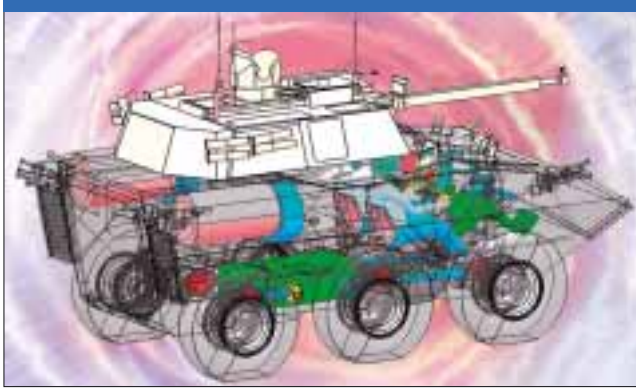
This study shows that a wheeled EB2X is also being considered. It features hybrid propulsion and a remotely operated turret. (Giat)
