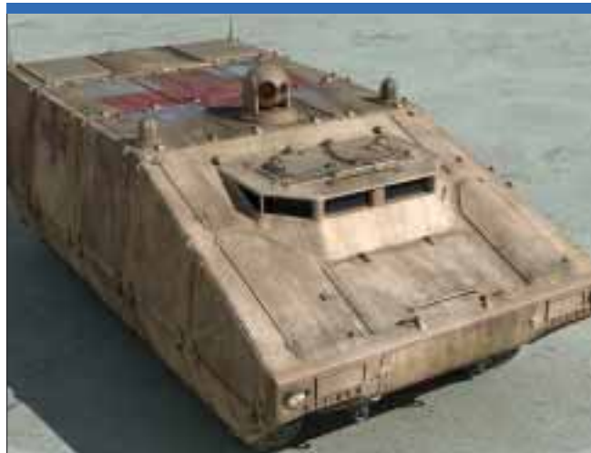
BAE Systems is leading the design and development of the Armed Robotic Vehicle. The ARV-RSTA (left) and the ARV-Assault ARV-A are designed to be controlled by troops on the ground or in manned ground vehicles. Under present plans each FCS brigade will include 45 ARVs. (BAE Systems)
