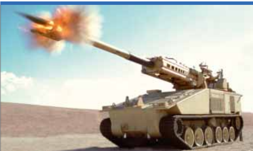
The BAE Systems 155 mm Non-Line of Sight Cannon (Nlos-C) is expected to be the first FCS Manned Ground Vehicle to enter service and Congress may put pressure on the army to further expedite the project in the wake of the Crusader cancellation. The concept technology demonstrator, mounting the M777's 39-calibre ordnance, passed the 1000 round milestone in mid-2005. (BAE Systems)
