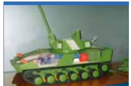
Wheels or tracks? Maybe both. This EB2X model features, inter alia, a hybrid powerplant (red generator at the back), a drone launcher, an active self-protection sensor atop the turret and a robot exiting via a rear-mounted ramp. (Armada/EHB)
