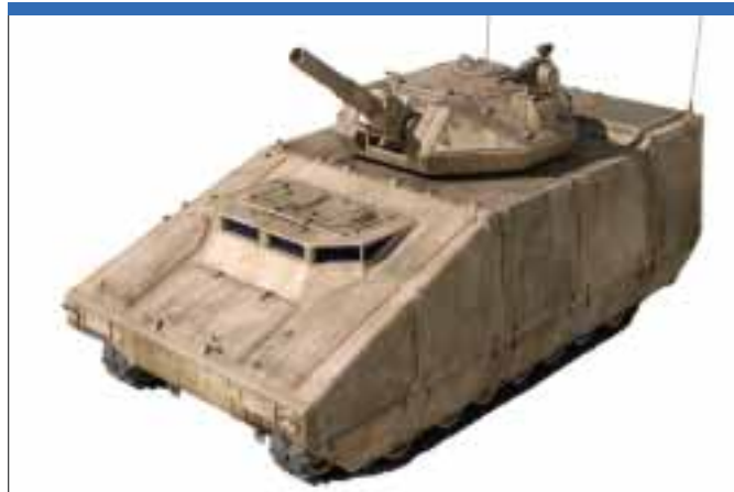
The BAE Systems Non-Line of Sight Mortar (Nlos-M) will be the first breech-loading 120 mm mortar in US Army service. Each will also carry an 81 mm lightweight mortar for dismounted operations. (US Army)
