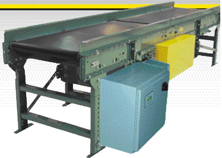
Four independent gap or pitch settings can be selected via discrete inputs to allow the required gap or pitch to be changed if requirements change. This feature was useful in one particular installation where the Gapper conveyor fed three print-and-apply applicators. The gap between products was dynamically selected based on the operational status of the 3 applicators.
