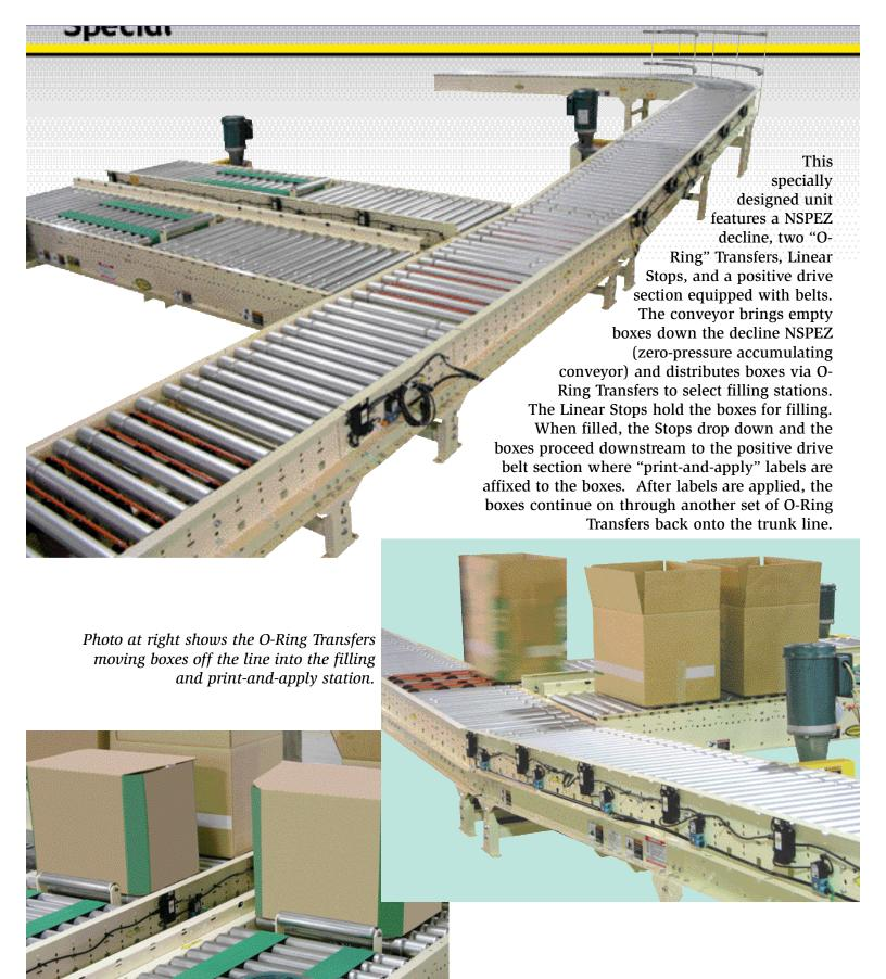
Linear Stops hold the boxes until the positive drive belt section is ready. Stops then drop down to allow the boxes to enter the belt section for labels to be applied.
