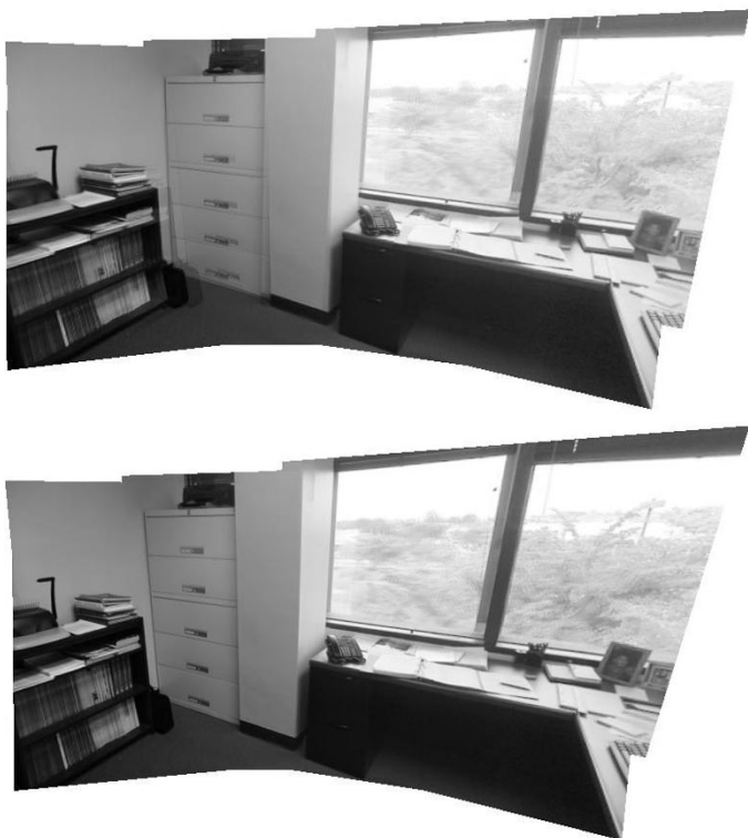
Fig. 5. Comparison between pair-wise and simultaneous joint registration of the "Office" sequence. The domain and range reference is the image in Fig. 4(a). Pair-wise registration results in misalignment noticeable around the file cabinet (top image) while simultaneous registration results in correct image alignment (bottom image).
