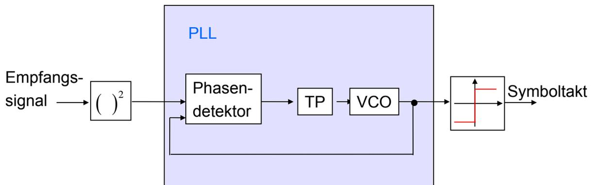
TP: Tiefpass; VCO: Voltage Controlled Oscillator
