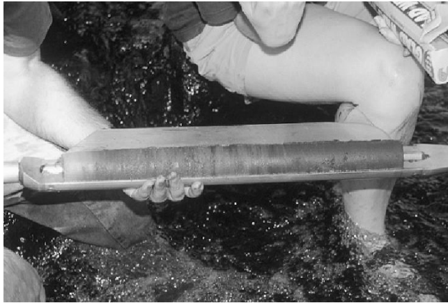
Figure 12. Pollen corer showing mud sample
