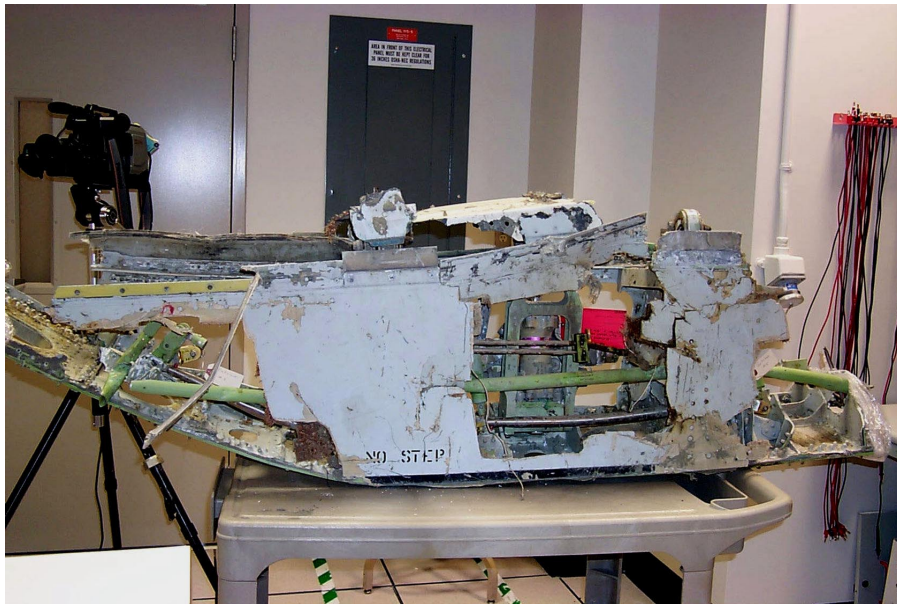
Figure 20 Right elevator center PCA attached to stabilizer rear spar
