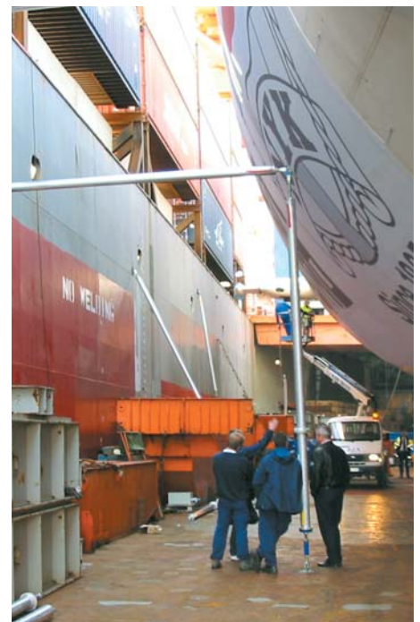
Zeppelin strapped down with aluminium fibre frames to vessel's deck and dockwall (portside).
