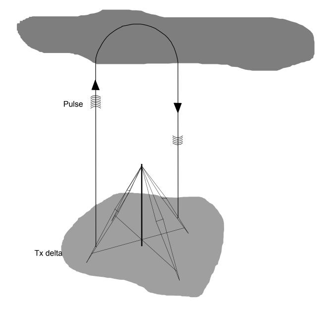
Figure 1.4 Ionosonde operation.
