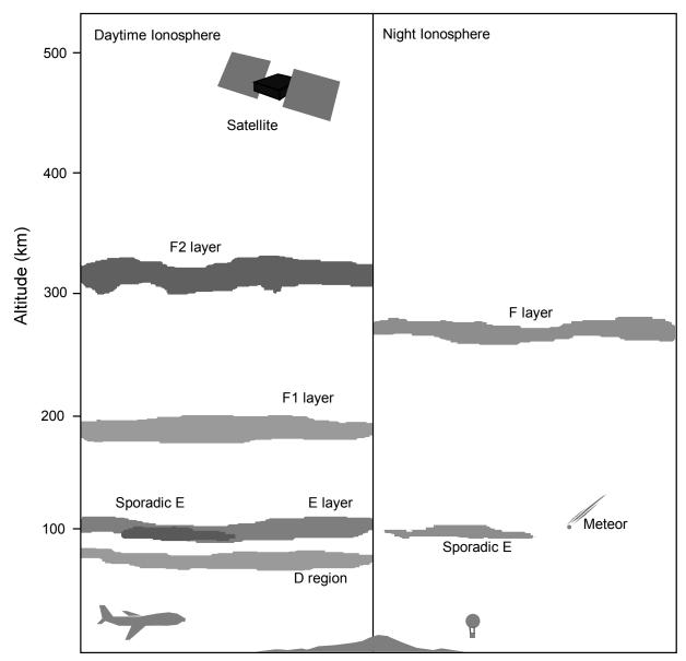
Figure 1.1 Day and night structure of the ionosphere.
