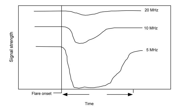
Figure 3.2 Fade-outs affect lower frequencies first and these are the last to recover. Higher frequencies are least affected and with many fade-outs will be unaffected.
