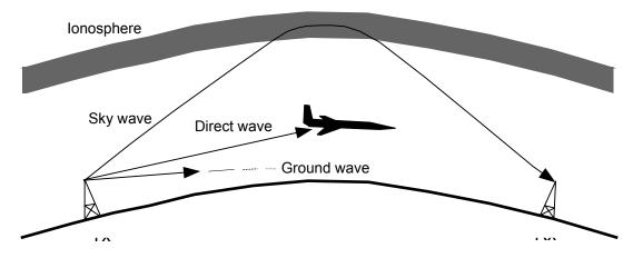
Figure 2.1 Types of HF propagation.
