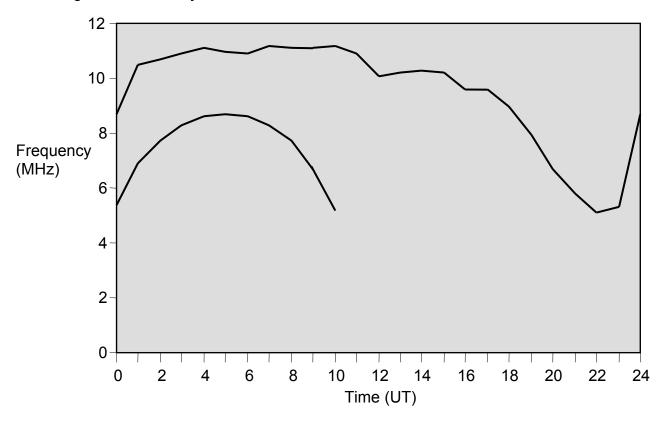
Figure 1.7 E and F layer frequencies for a Singapore to Ho Chi Minh circuit sometime in a solar cycle.
