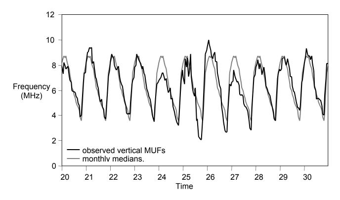
*Figure 3.3 Canberra, Australia observed and median vertical MUFs for the latter part of September 1998. Significant depressions in F region frequencies occurred between 24 to 28 September due to solar activity.*
