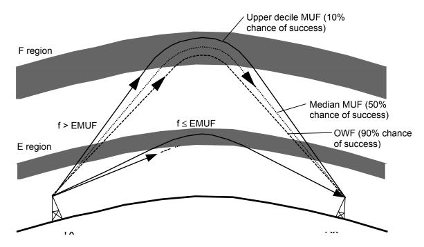
Figure 2.2 Range of usable frequencies. If the frequency, f, is close to the ALF then the wave may suffer absorption in the D region. If the frequency is above the EMUF then propagation is via the F region. Above the FMUF the wave is likely to penetrate the ionosphere.
