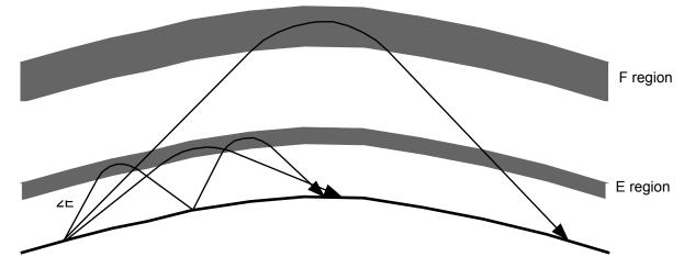
Figure 2.4 Examples of simple propagation modes.
