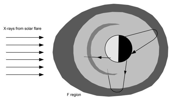
Figure 3.1 Fade-outs affect only those circuits where the wave passes through the D region. That is, circuits with daytime sectors. Night circuits are unaffected by fade-outs.
