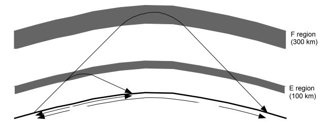
Figure 2.3 Hop lengths based upon an antenna elevation angle of 4° and heights for the E and F layers of 100 km and 300 km, respectively.
