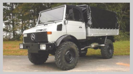
• The cheapest modification to the basic Unimog 1700L/38 and 2450L trucks would be the retrofit of a 'convertible' cab. A proven design exists in the U1300L soft top production variant.
