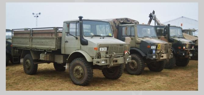
• A range of Unimog 1700L/38 configurations are in use. The height of the Unimog hard top cabin is the only impediment to loading Unimogs via the Nose Cargo Door of the KC-33A.
